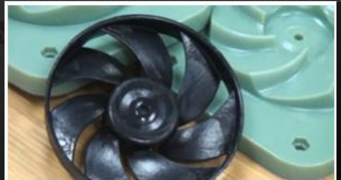
Engine cooling fan made from POM (acetal) using a Stratasys 3D printed injection mold
