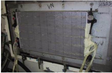
Figure 15: Radiator mounted on test bench.
