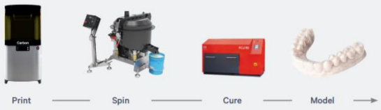
Workflow from Resin to Models in Less than an Hour
