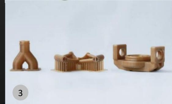
PEKK/PEEK 3D打印零件举例
